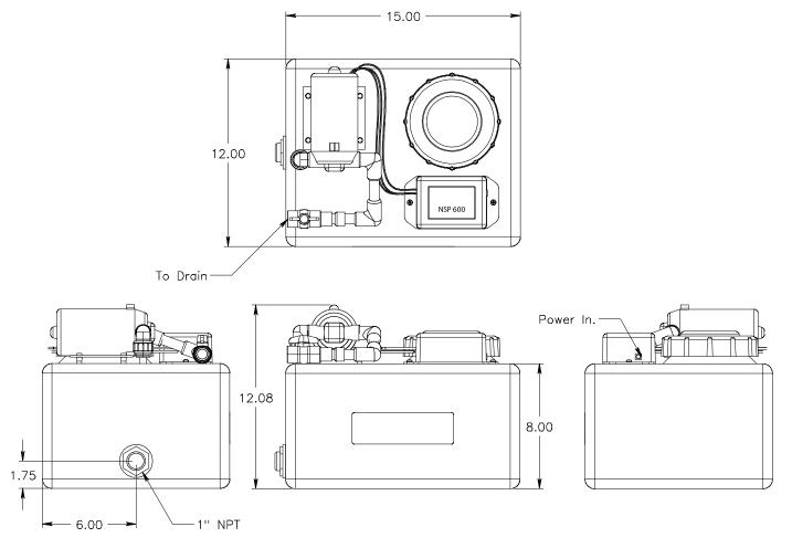
This combination condensate neutralizer and condensate pump features:
