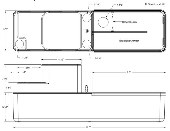
This combination condensate neutralizer and condensate pump features a Little Giant model VCMA-20ULS pump assembly mounted to Neutra-Safe's patent pending serpentine flow neutralizing base.
