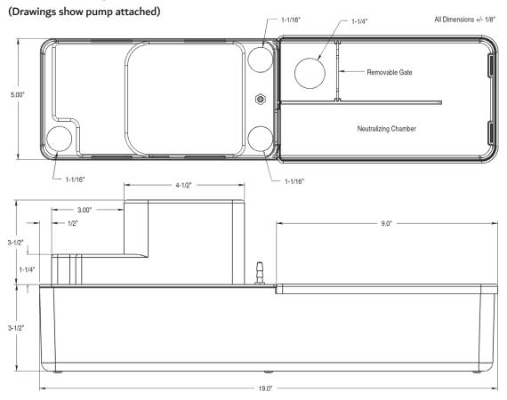
This condensate neutralizer pump base enables a VCMA Little Giant pump assembly to be mounted to Neutra-Safe's patent pending serpentine flow neutralizing base. Pump simply unsnaps from Little Giant base and snaps on to the Neutra-Safe base.
