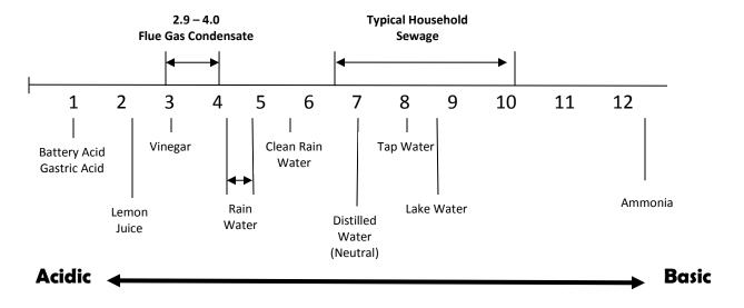
Treated condensate should be as close to neutral as possible with 5 being the minimum. Most national and state codes <sup>1</sup> prohibit anyone from allowing acidic liquid into a drainage system without treating it to raise its pH.
